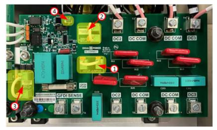
Figure 4: 30C3-CE DC2 and DC3 Connect Board
