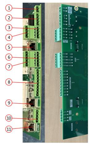
Figure 1: Control Board Low-Voltage Connectors
