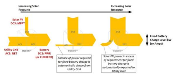
Figure 6: Three port power flow example with utility grid at AC1 as = NET
